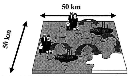
Figure 4. Flow of nitrogen load within a grid cell from the human population via sewage treatment to natural wetlands. The white area represents the natural wetland area within a grid cell.
