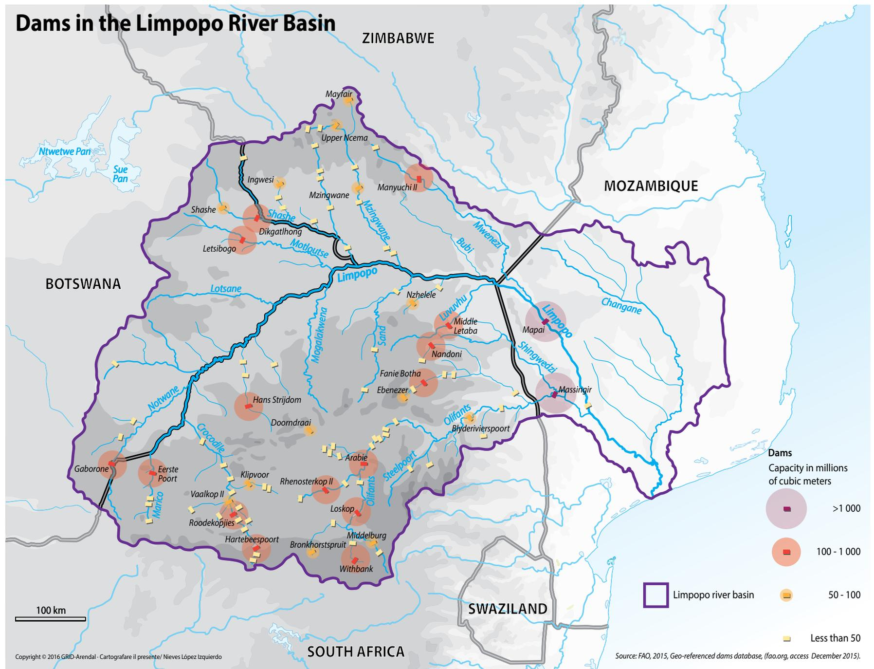
**Figure 2.17 Dams With a Storage Capacity of More than 30 Million Cubic Metres and Related Bulk Infrastructure for Water Supply in the Limpopo Basin**
