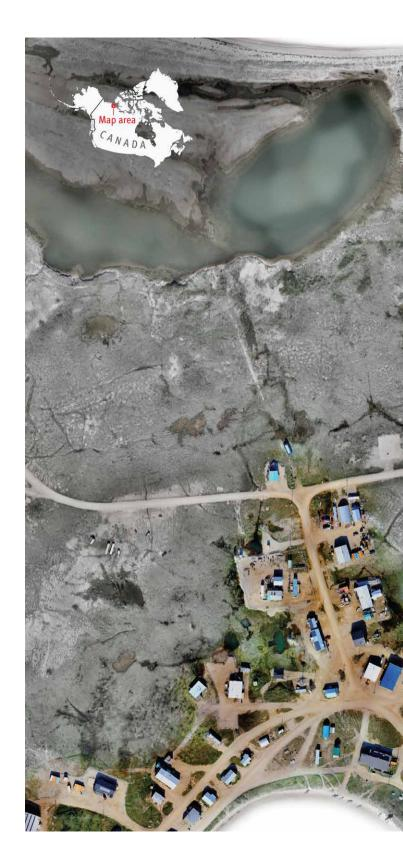
Paulatuk's airport is built on permafrost, with sand and gravel elevating it about 2 metres above the ground. The runway is located less than 100 metres from the shoreline facing the Amundsen gulf. It has experienced rapid erosion up to 80 centimetres per year.
