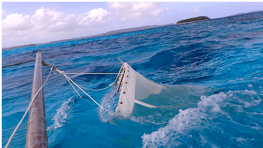
Fig. 3. The phytoplankton net position in the water during sampling.
