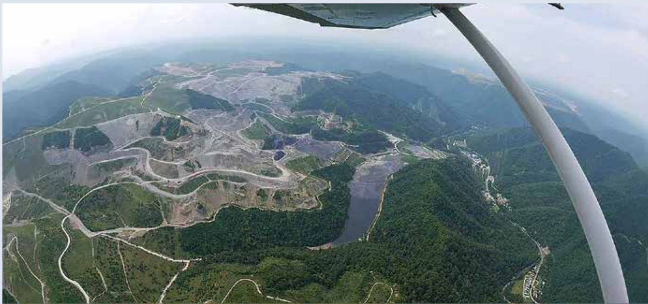
The top has been blasted off this mountain ridge in South Western Virginia and a large dam constructed to store sludge waste. Photo © OVEC/Vivian Stockman
