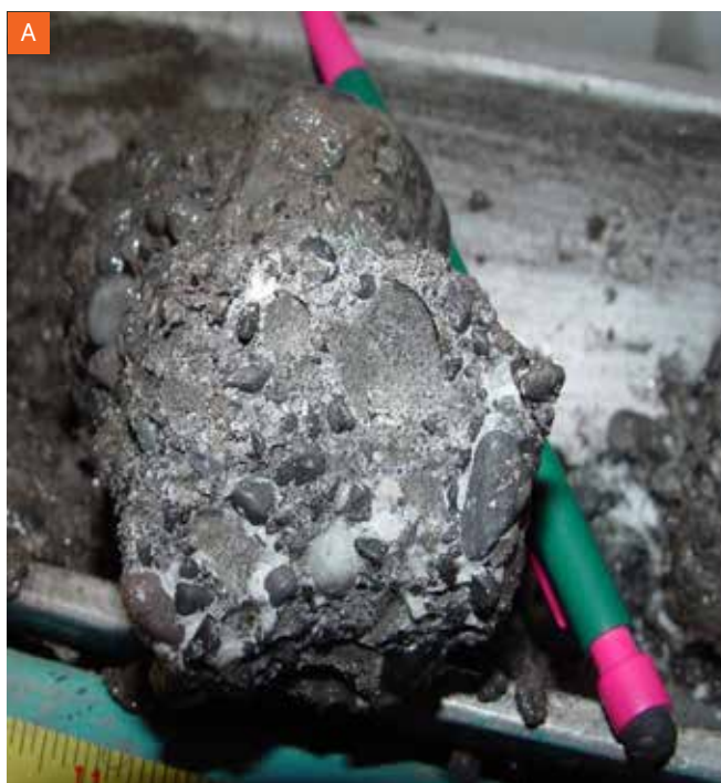
In sands and other coarse-grained sediment, gas hydrate (white) can form between the sediment grains (dark grains) as shown in this example from the Canadian Arctic.
