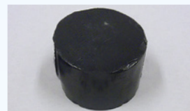
Solidification as sulphur polymer.
