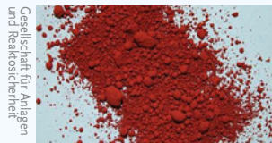
Solidification as mercury sulphide.
