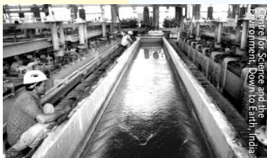
An open mercury-cell at a chlor-alkali plant.
