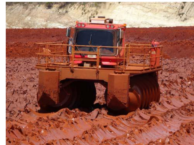
Figure 5. Amphirol or scroller on red mud
