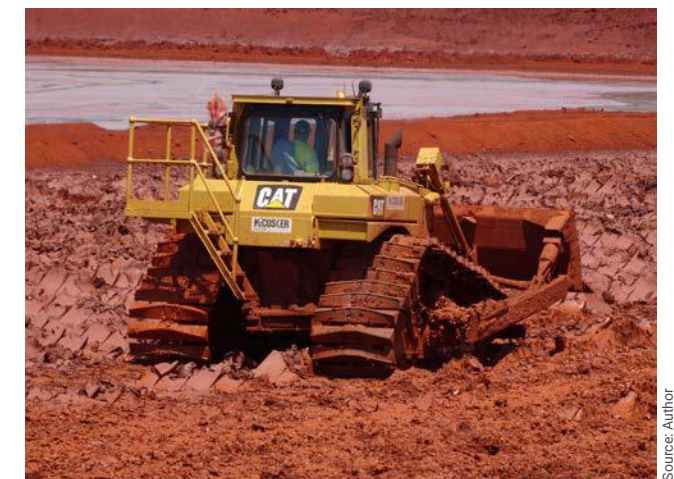
Figure 6. D6 Swamp Dozer on red mud
